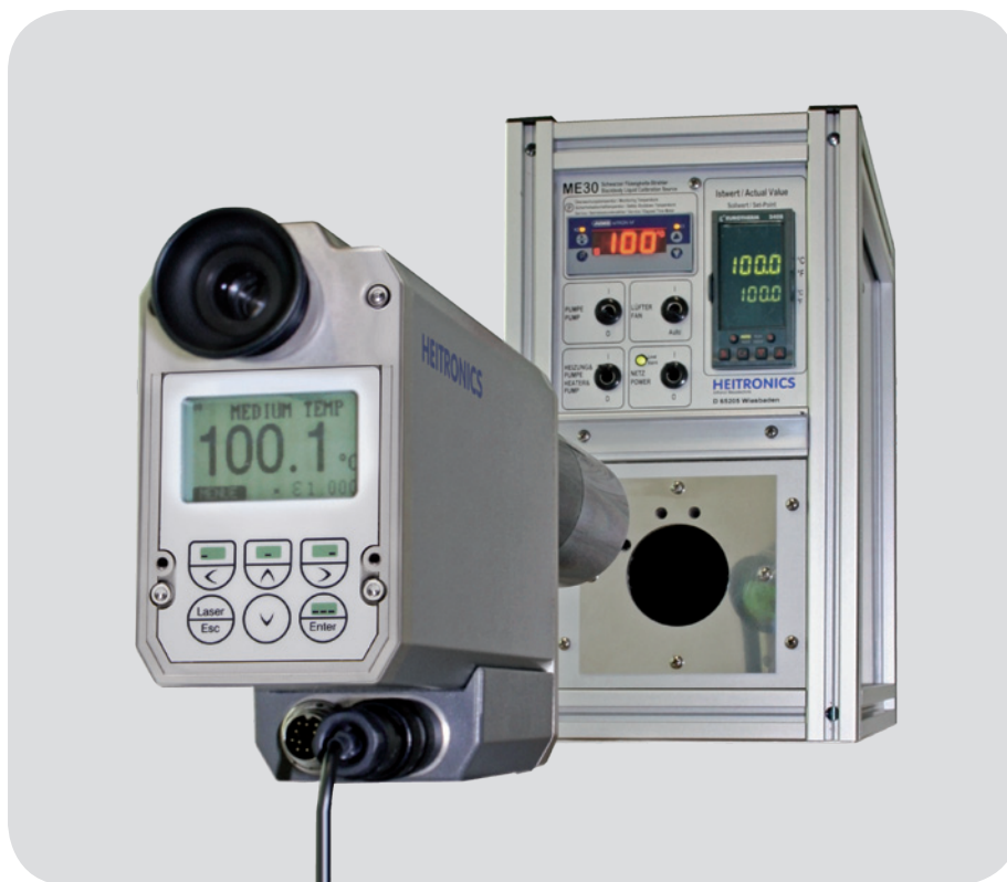
Figure 2: Calibration of ME30 with Transfer Radiation Thermometer (TRT)
